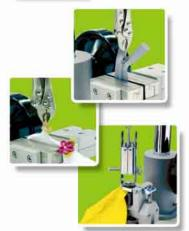
**SafGuard** is a patented safety test instrument that provides a means to accurately measure how safe accessories are attached in a product.
