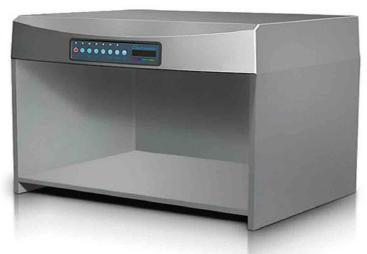
Colors appear differently under different lighting sources. To avoid or reduce the assessment error when performing color contrast, we can use a Light Booth (aka: Viewing Booth, Light Box) to simulate different light sources to obtain an objective assessment of color and color difference anytime anywhere.
