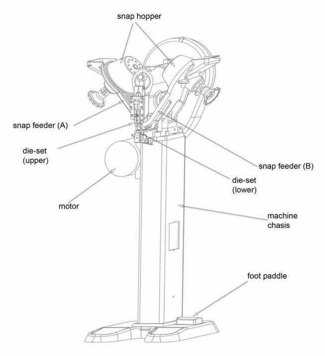
NOTE: Typically two machines are required to complete a full set of press fastener. One machine is for attaching Part 1 (Cap & Stud)" and another machine is for Part 2 (Socket & Post)". Only one fixed size of snap can be attached. Using other types or sizes of snap will cause machine malfunctioning and machine will not work properly.
